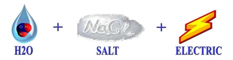
To produce one liter of the disinfection solution we need 2-4 gram of slat and 4-5 watt
